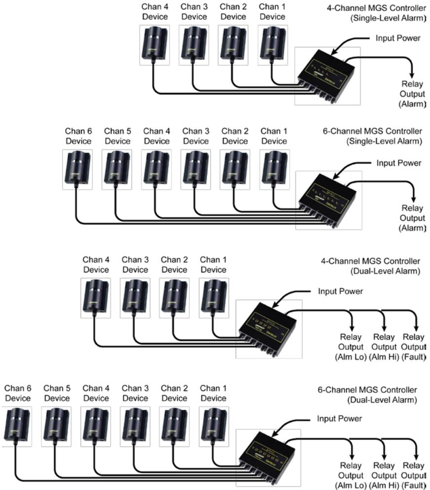
**Figure 2. Sample Configurations (4,6-Channel)**
