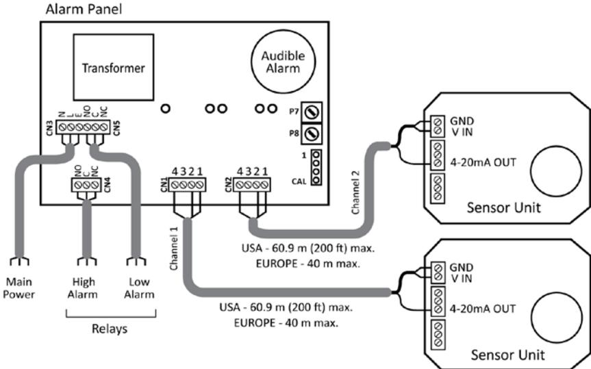
**Figure 9. Wiring (2-Channel, Dual-Alarm Unit Shown)**
