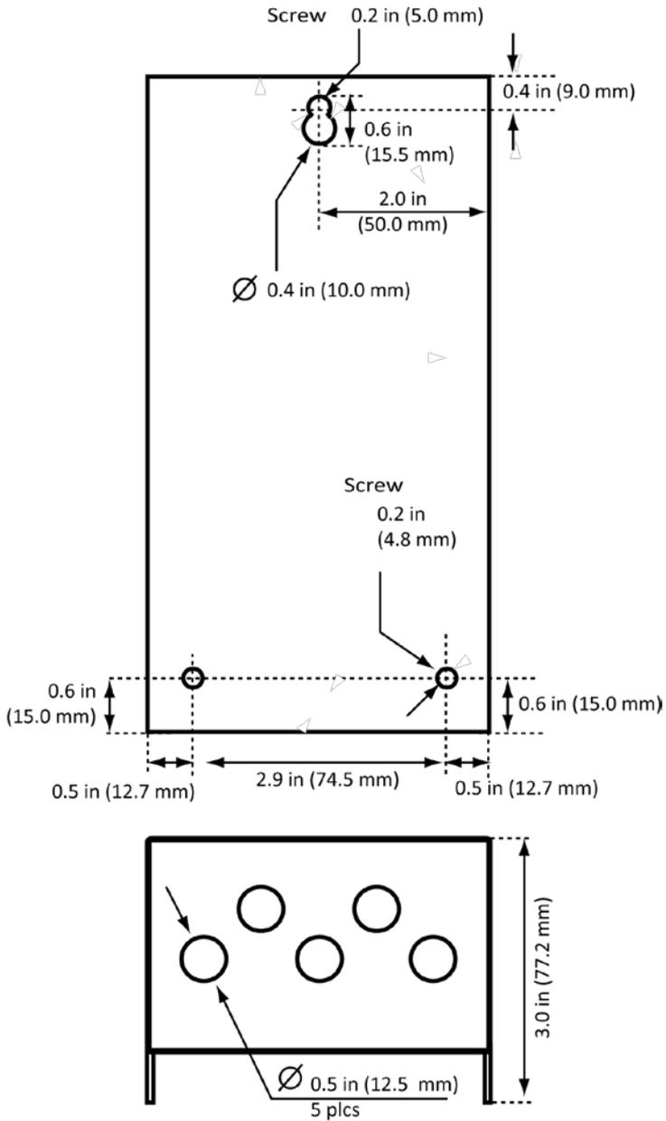
Figure 6. Mounting Dimensions (2-Channel Unit)
