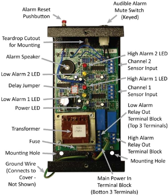
**Figure 5. 2-Channel, Dual-Alarm MGS Controller**
