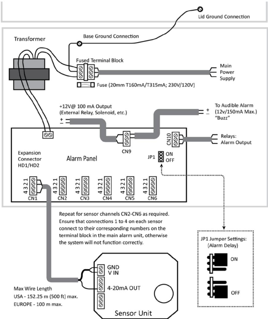
**Figure 10. Wiring (6-Channel, Single-Alarm Unit Shown)**
