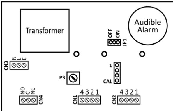
Figure 12. Hardware PCB Layout (2 Channel, 1 Alarm)
