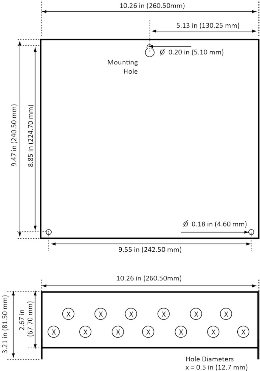
**Figure 7. Mounting Dimensions (6-Channel Unit)**
