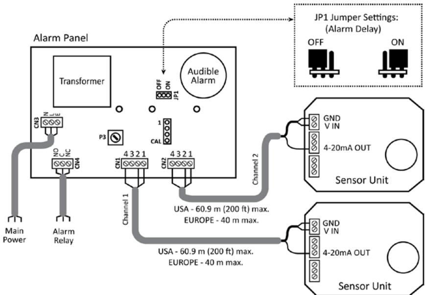
Figure 8. Wiring (2-Channel, Single-Alarm Unit Shown)
