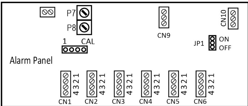
**Figure 15. Hardware PCB Layout (6 Channel, 2 Alarm)**
