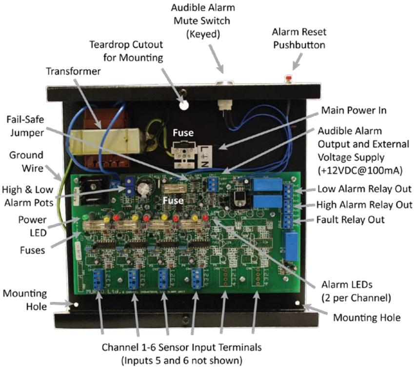
**Figure 4. 6-Channel, Dual-Alarm MGS Controller**
