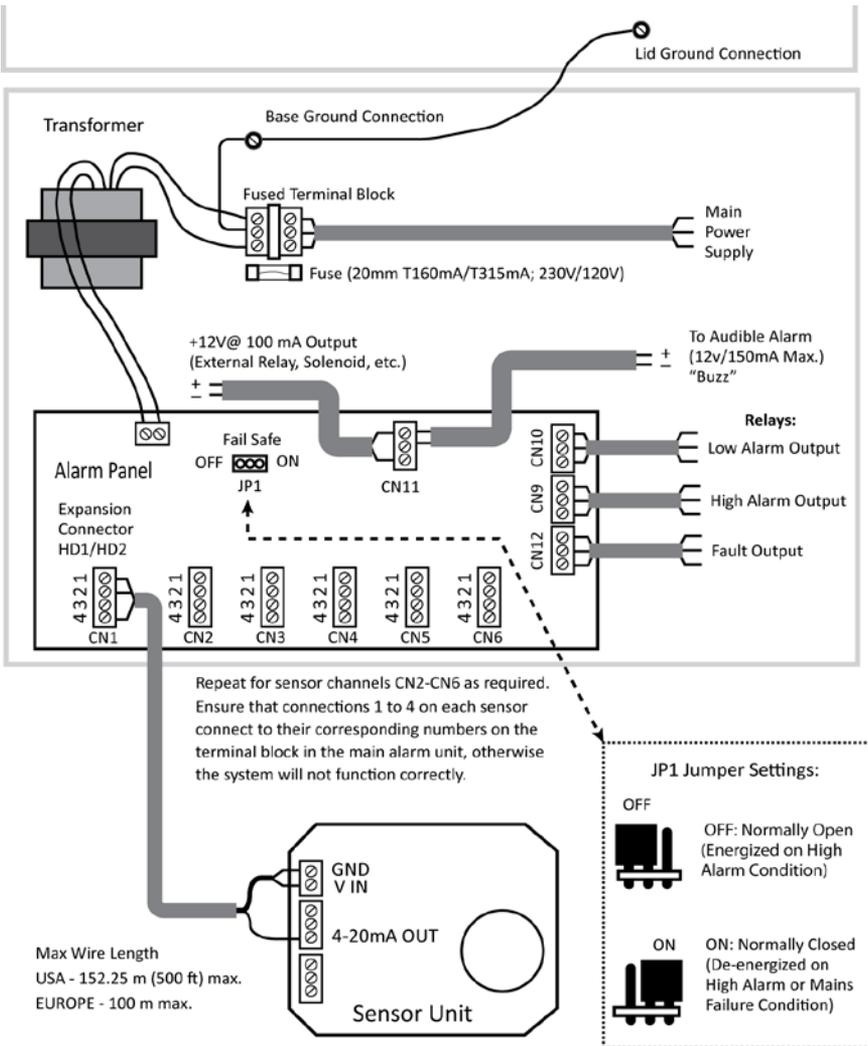
Figure 11. Wiring (6-Channel, Dual-Alarm Unit Shown)
