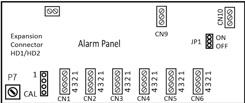
**Figure 14. Hardware PCB Layout (6 Channel, 1 Alarm)**
