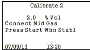
Figure 5-6: Mid-Span Gas Calibration
