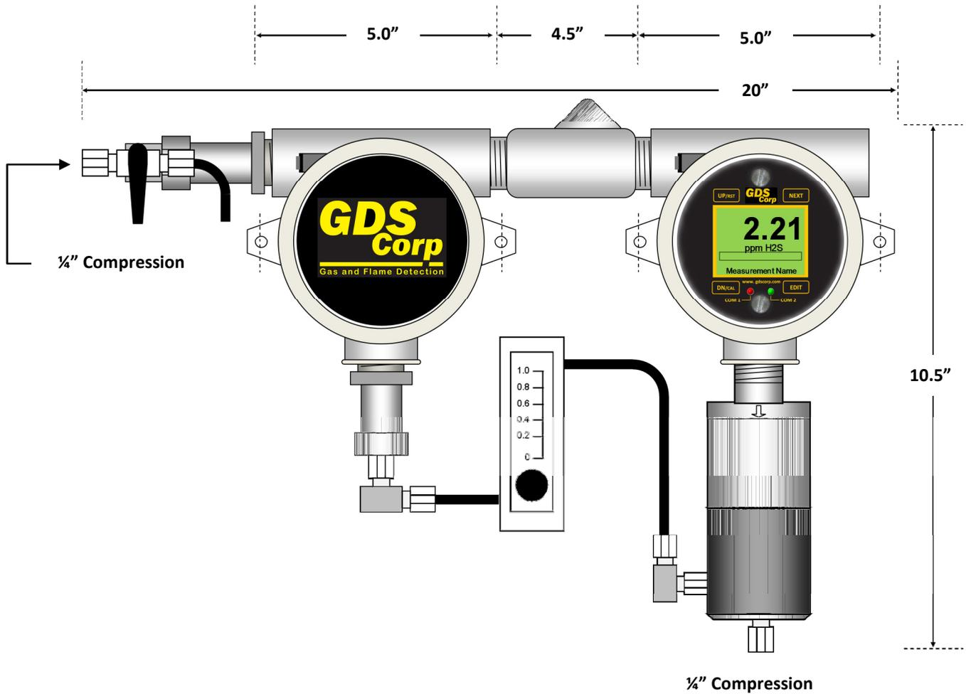
Figure 13-1: GDS-58NXP Dimensions (Aluminum Enclosure)
