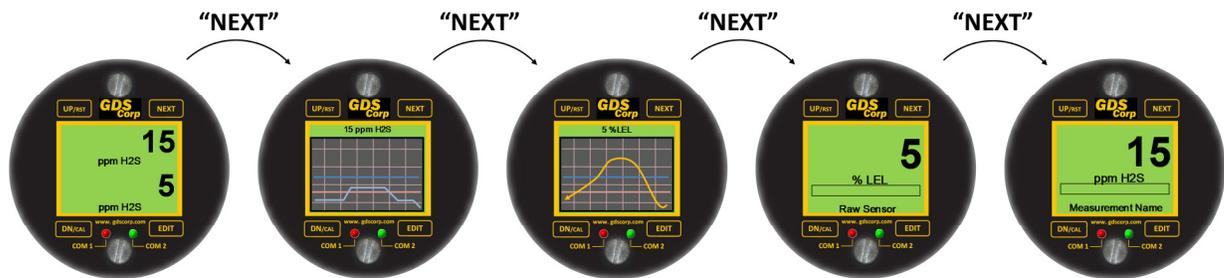
Figure 5-3: Dual Channel Display Sequence
