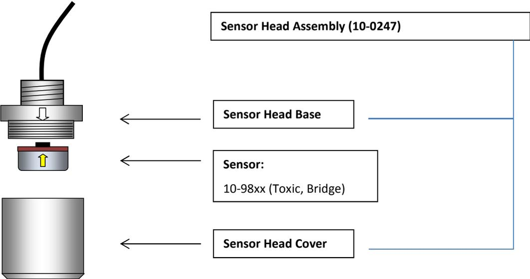
Figure 12-2: GDS-58NXP Standard Sensor Head Exploded View
