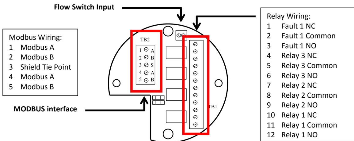
**Figure 4-2: RELAY / MODBUS Connections**
