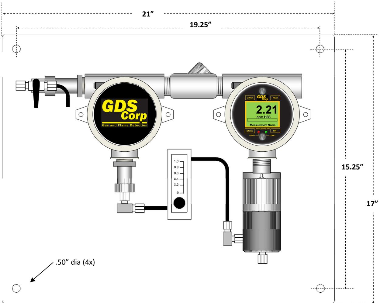
Figure 13-4: GDS-58NXP 21" x 17" Mounting Plate Dimensions
