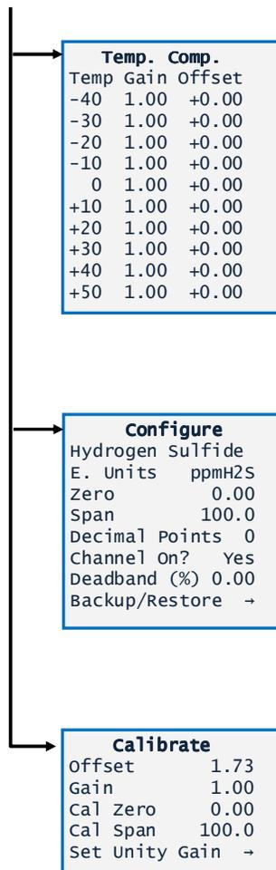
**Temperature Compensation** compensates for changes in sensor output (gain) and zero value (offset) as sensor temperature changes. Individual values for gain and offset can be entered for eleven points ranging from minus 40C to +60C. Gain and offset values are linearly interpolated between points by the internal microprocessor.
