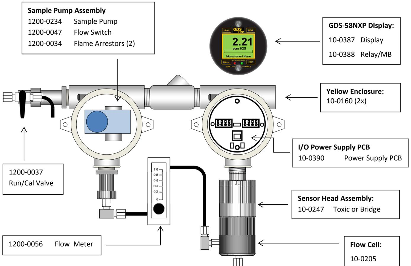
Figure 12-1: GDS-58NXP Assembly with Toxic / Bridge Sensor (Spare Parts)
