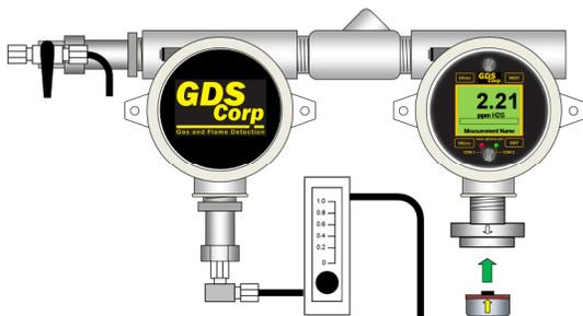
Step 6: Install the new sensor by aligning the arrow on the sensor with the arrow on the sensor head and push straight up.
