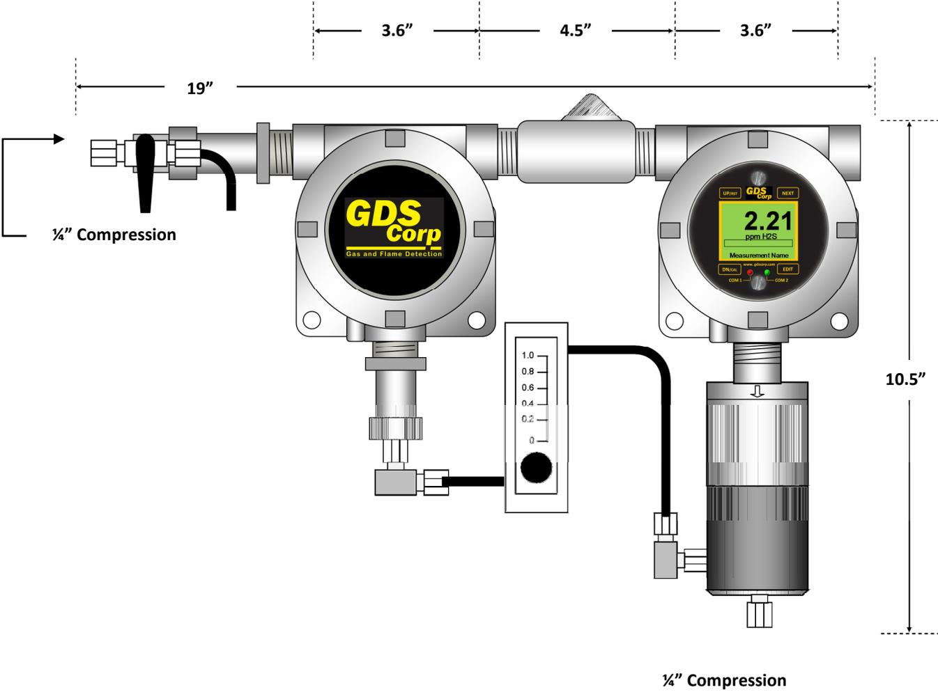
Figure 13-2: GDS-58NXP Dimensions (Stainless Steel Enclosure)
