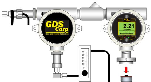
Step 4: Pulling straight down, remove the existing sensor.
