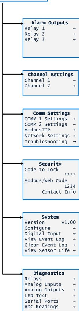
**Alarm Output Menu** – contains settings that control the four optional alarm relays (if installed). These setting include relay programming, on and off delay, failsafe mode and specific input override.
