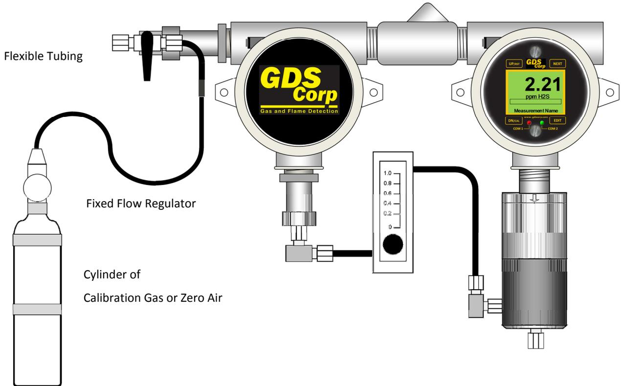
Figure 6-1: GDS-58NXP Calibration Setup
