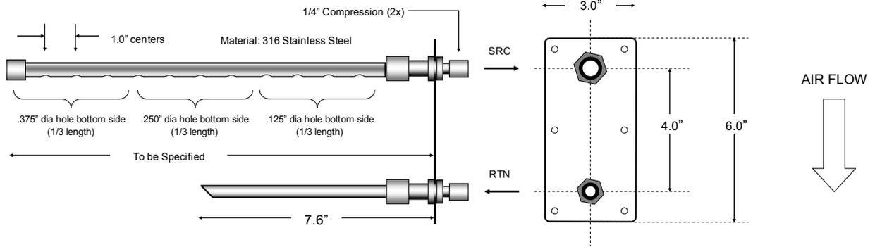
Figure 15-1: Sample Draw Duct Assembly
