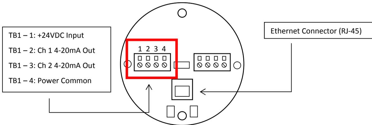
**Figure 4-1: GASMAX CX I/O Board**
