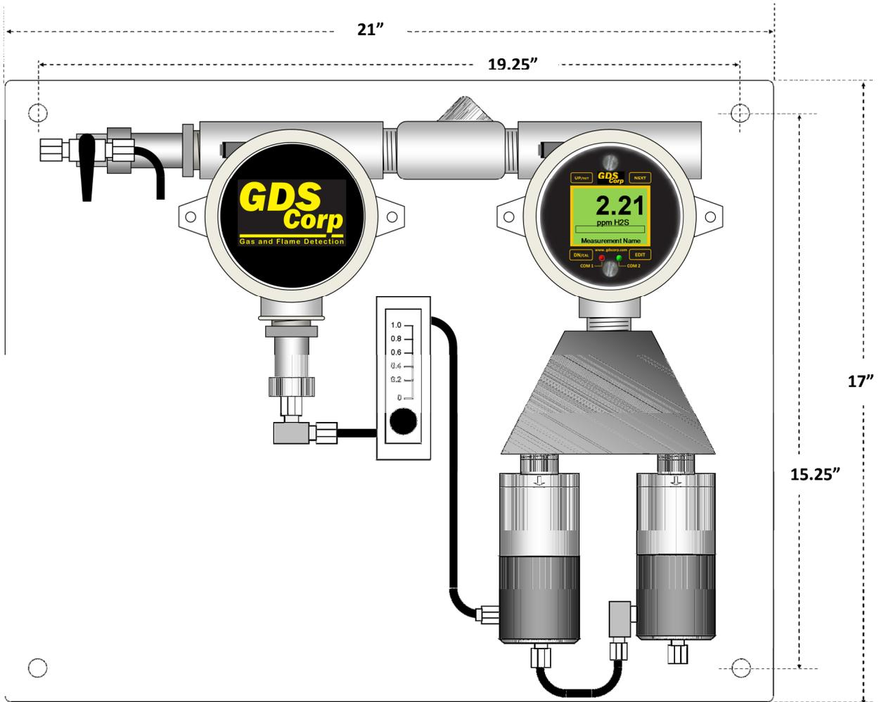
Figure 13-5: GDS-58NXP 21" x 17" Mounting Plate (Dual Sensor)
